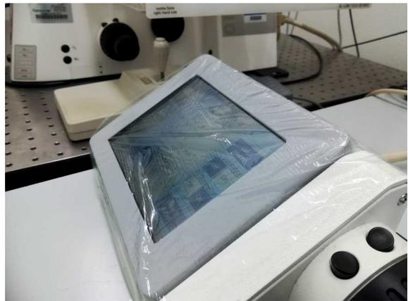
Microscope eyepieces, touchscreen, computer keyboard and mouse wrapped in cling film, to create a disinfectable surface.
